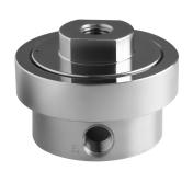
Premier 2400DL series dome loaded, low pressure, high flow, back pressure regulators are fitted with a large Viton® diaphragm for increased sensitivity. These precision, back pressure regulators feature a cracking pressure of 0-75 PSIG (0-5.17 bar), 1.3 to 1 dome load, and Cv 0.6. Premier 2400DL series regulators are capable of regulating a broad range of media as compatible with their materials of construction.
