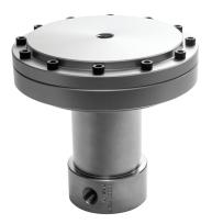
Premier SCF 3123AL Series high pressure, air loaded, back pressure regulators are elastomer free, designed to stand up to the aggressive, solvent-like qualities of supercritical CO2, while providing reliable and precise pressure regulation. These single stage, piston sensed regulators are designed for inlet and outlet pressures up to 15000 PSIG (1034.21 bar) and Cv 0.06.
