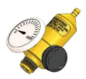
Economical, piston sensed, fixed flow, pressure reducing regulators used for calibration gases and industrial hygiene monitors. Premier 2700E Series regulators are set using a unique integrated flow adjustment valve prior to shipment; flow settings range from 0.25 LPM to 9.0 LPM. Premier 2700E Series regulators are rated for inlet pressures up to 1500 PSIG (103.4 bar).
